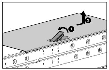
Figure 1-4: Removing the access panel
